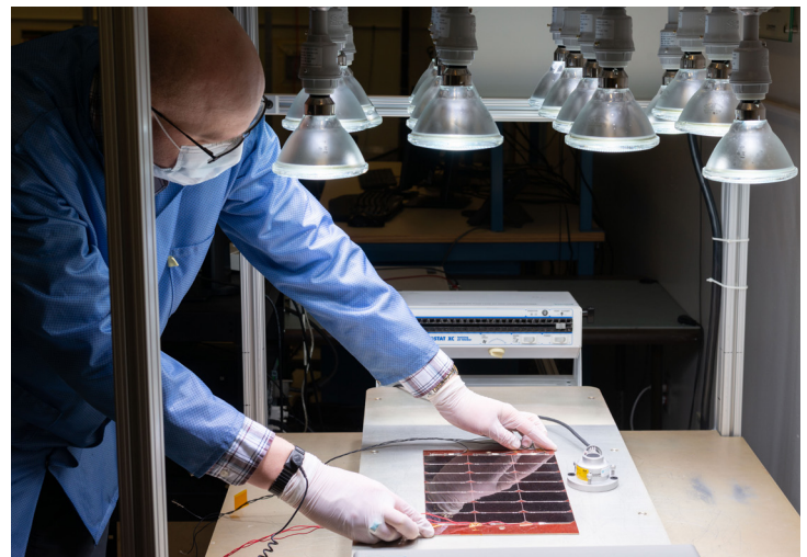
Solar panel illumination at the solar simulation station.
