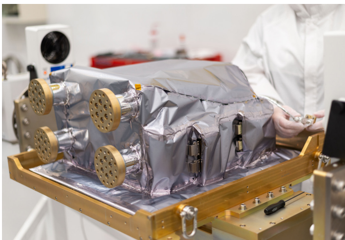
Assembled flight SDA covered with protective multi-layer insulation (MLI) blanketing.
