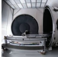
Thermal Vacuum Testing (large)
