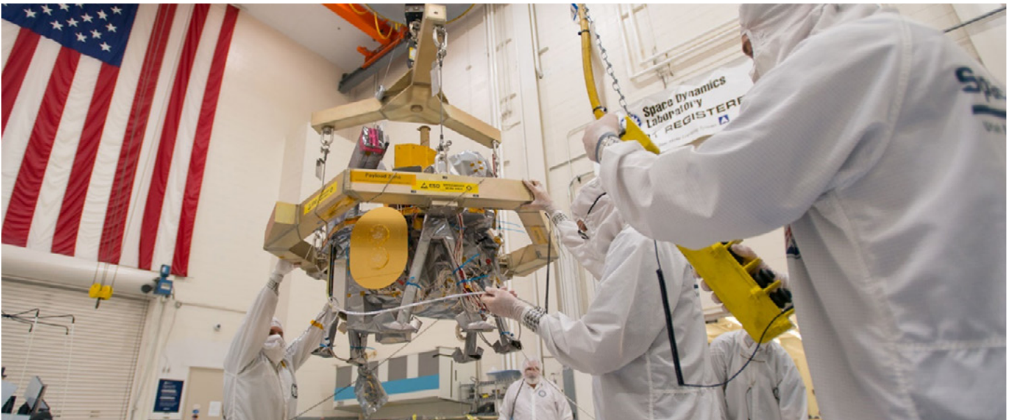
ICON payload I&T at SDL facilities in North Logan, Utah.
