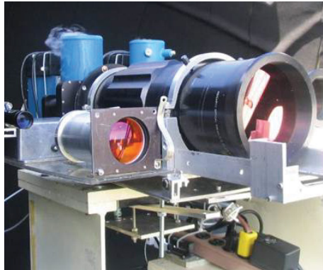
Two Santa Barbara Focalplane infrared cameras were used to collect high-speed imagery (>2,000 fps) of a rocket launch at Kennedy Space Center.
