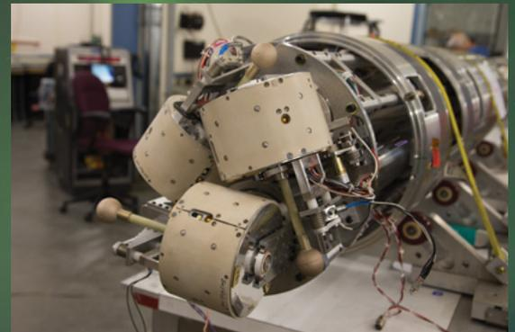
*Three aft sub-payloads being integrated into the rocket body. The sub-payloads are spun to 2 Hz in their cradles and ejected using pneumatic pistons at high velocity. Each sub-payload was ejected from the rocket at 50 m/s in different directions to create a network of measurement points.*
