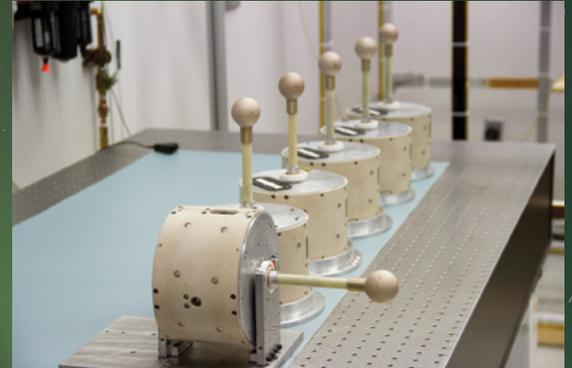
*Six flight sub-payloads shown in SDL's SmallSat Verification and Validation Laboratory after static balance testing. The payload consists of three science instruments, with GPS and communications hardware tightly integrated in a 6" diameter cylinder.*
